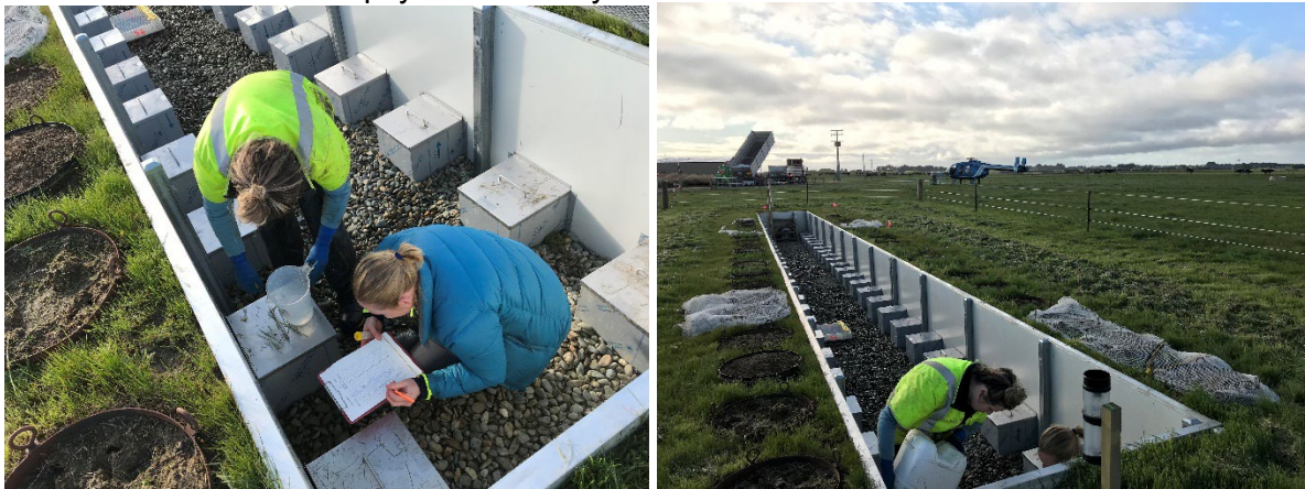
Figure 9: Leachate sampling from the Plant & Food lysimeters
